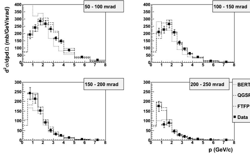
Figure 1. Double differential cross sections of  $\pi^+$  forward production by 12 GeV/c protons off thin Carbon target: histograms – Geant4 9.3p01 simulation (BERT, QGSP, FTFP), points are data (Catanesi et al. 2008).
