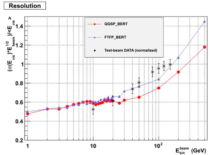
Fig. 2. Energy resolution for a sampling copper-liquid argon calorimeter. The resolution is shown as a function of the beam kinetic energy for impinging negative pions. The data from ATLAS-HEC test-beam are compared to the predictions of QGSP\_BERT (red) and FTFP\_BERT (blue) physics lists. Simulations obtained with GEANT4 version 9.5. $\beta$  (June 2011).
