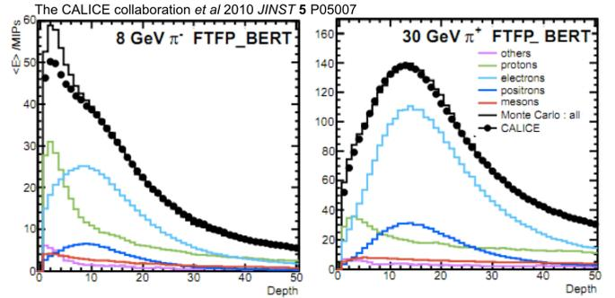
Fig. 7. Longitudinal profile obtained by the CALICE collaboration with the test-beam data of a tungsten, silicon digital calorimeter. Pions beam with two energies are shown: 8 GeV (left) and 30 GeV (right). The simulation is obtained with GEANT4 version 9.3 and the FTFP\_BERT physics list. For the simulation the contribution to the shower profile of each particle species in the profile is also shown. Courtesy of the CALICE collaboration [5].
