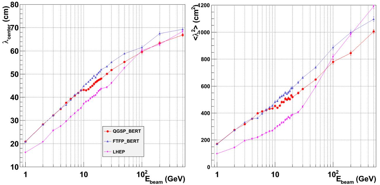
Fig. 5. Simulation of pion induced showers in an iron-scintillator calorimeter obtained with GEANT4 version 9.5.β. The shower depth (left) and shower length (right) of three different physics lists (LHEP , FTFP\_BERT , QGSP\_BERT ) are compared.
