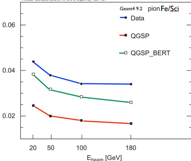
Fig. 3. Lateral leakage for the Tile calorimeter. The ratio between the energy released in the module displaced with respect to the beam axis and the central module is shown as a function of beam energy. The modules are about 30 cm wide. Test-beam data are in blue, QGSP\_BERT is shown in green and a physics list without a cascade model is shown in red.
