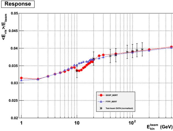
Fig. 1. Ratio between energy released in the active material and beam energy for a sampling copper-liquid argon calorimeter. The ratio is shown as a function of the beam kinetic energy for impinging negative pions. The data from ATLAS-HEC test-beam are compared to the predictions of QGSP\_BERT (red) and FTFP\_BERT (blue) physics lists. Simulations obtained with GEANT4 version 9.5. $\beta$  (June 2011).
