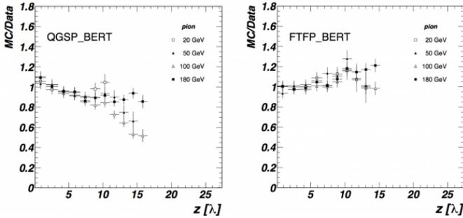
Fig. 6. Monte Carlo-data ratio for the energy deposit as a function of the shower depth. Left: simulations obtained with the QGSP\_BERT physics list; right: simulations obtained with the FTFP\_BERT physics list. Courtesy of the TileCal collaboration [12].
