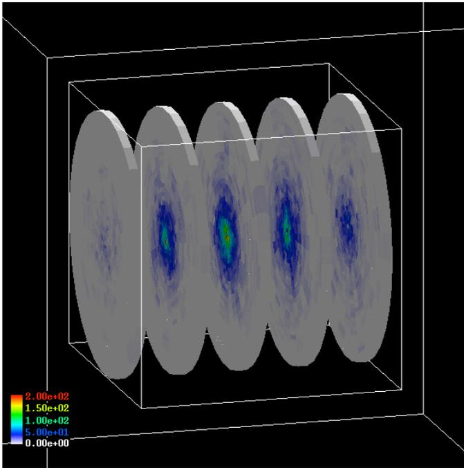
Figure 2. Example of a cylindrical scoring geometry embedded inside a large water volume. The scoring geometry is created at runtime, in a separate parallel geometry. No checking for overlaps with the ‘material’ geometry is required as a consequence.
