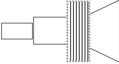
Figure 1. Picture of a simple setup with 2 parallel geometries: the ‘material’ geometry of two boxes and a trap overlaid by the mesh for scoring radiation flux. The scoring geometry must be separate and parallel, as it occupies the same space. Otherwise it would cause overlap errors.
