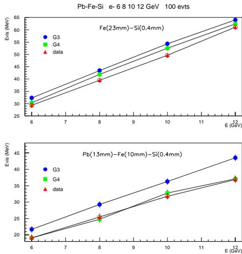
**Figure 1:** Visible energy versus incident energy: data from [9], Geant3 and Geant4 simulations.
