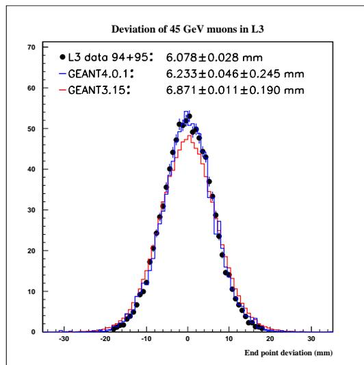
**Figure 3:** Deviations of 45 GeV  $\mu$  in L3: experimental data, Geant3 and Geant4 simulations.
