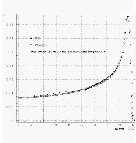
**Figure 2:** Comparison between Geant4 simulation and experimental data for medical applications
